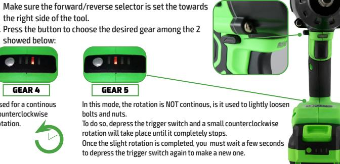
Used for a continuous counterclockwise rotation.
